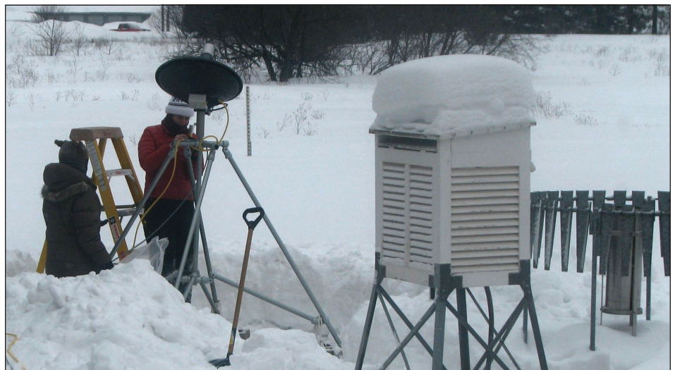
Graduate students Claire Petterson and Elin McIllhattan put the final touches on the Micro Rain Radar setup at the Marquette Weather Forecast Office.
